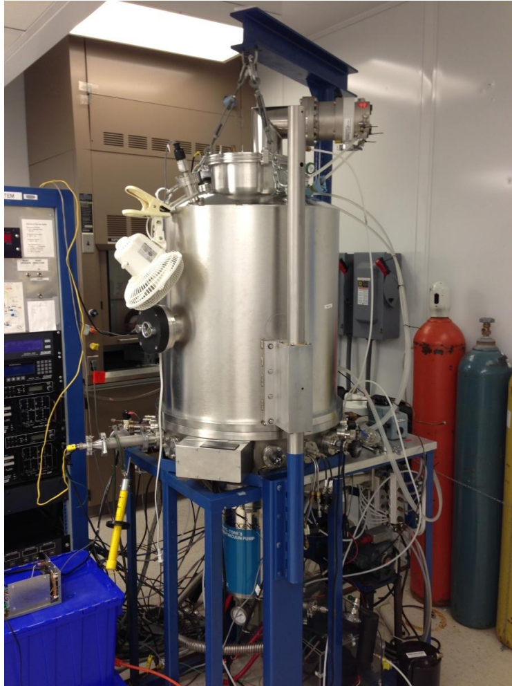
Figure 3-4 The EBPVD system is picture here. The vacuum chamber can be seen at the center. The cryopump is beneath the chamber and capable of the pumping the system down to a base pressure of under 3E-6 Torr.
