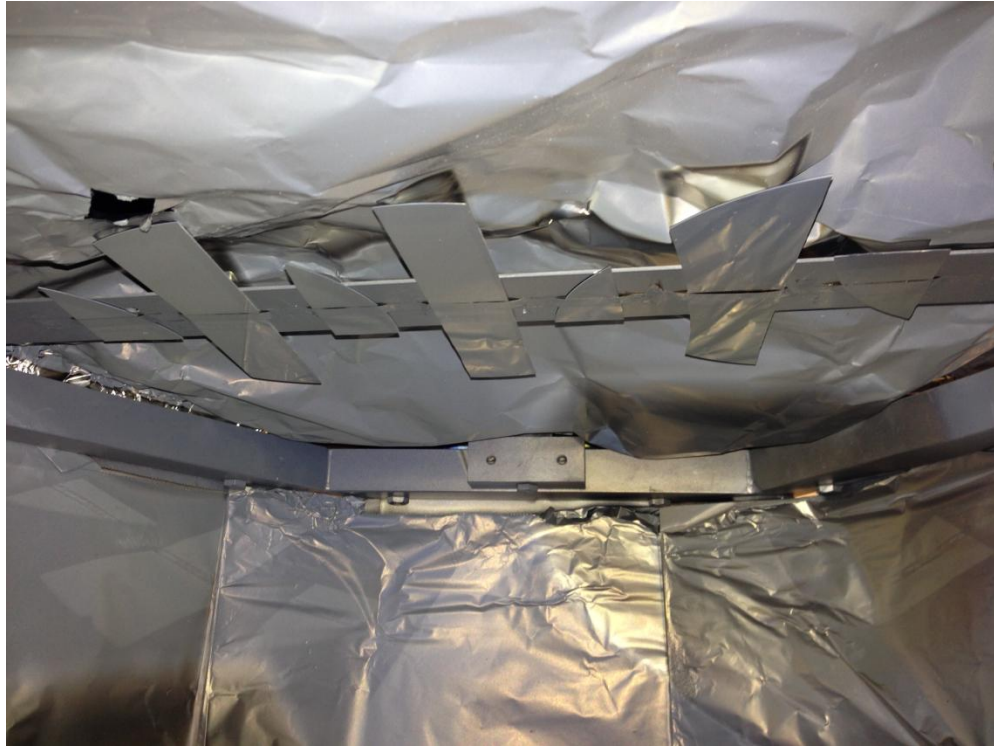
Figure 3-3 This picture shows the positioning bar within the chamber immediately after a deposition. The bar covers nearly the entire width of the chamber and as a result a gradient of composition, deposition rate, and thickness is achieved in a single run.
