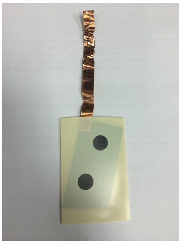
Figure 3-12 Thin film prepared for electrochemical testing. Multiple test areas were able to be placed on a single thin film. The electroplating tape acts as a mask so that only the exposed area is tested. The copper tape provides electrical contact to the surface of the thin film.
