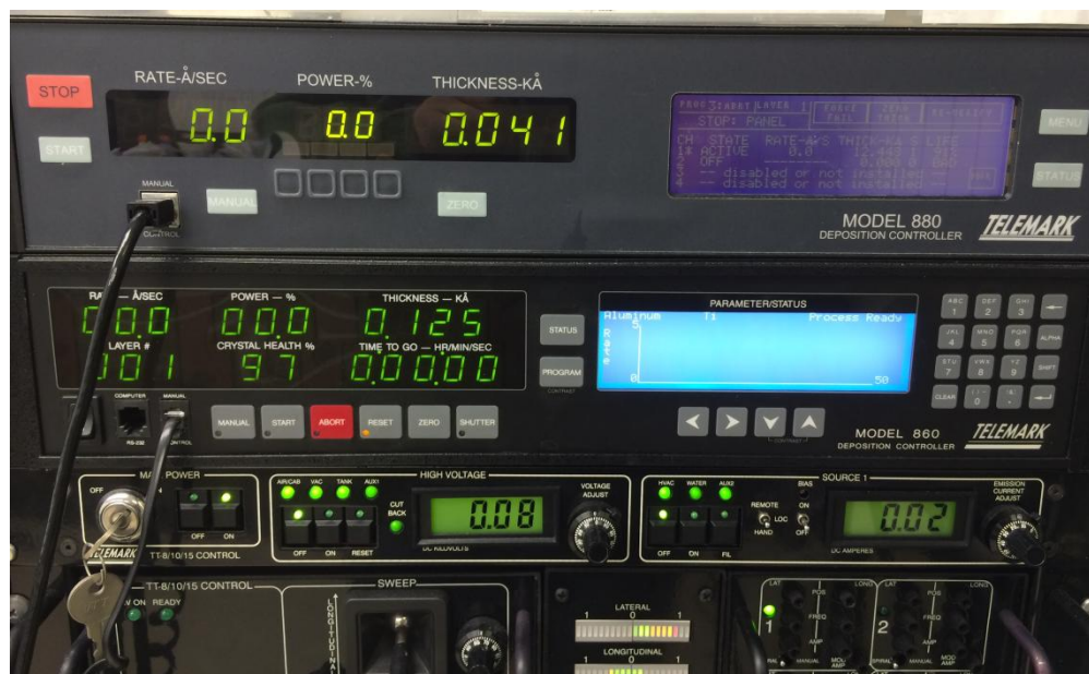
Figure 3-5 Deposition controllers for the EBPVD system. The Telemark Model (top) and the Telemark Model 860 (bottom) are both capable of controlling the power transferred to the electron guns, the deposition rate (by varying the power), and measure rate and thickness using quartz crystal microbalances within the chamber.
