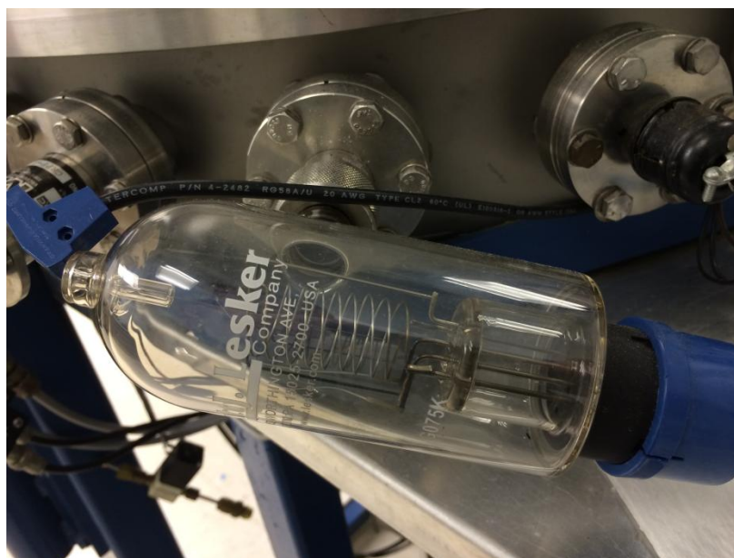
Figure 3-6 Kurt J. Lesker G075K ion gauge is used to measure the pressure in the chamber during deposition.
