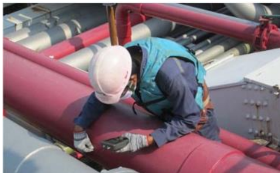
Figure 1.5: NDE of a pipe section using a hand held ultrasonic transducer [45]
