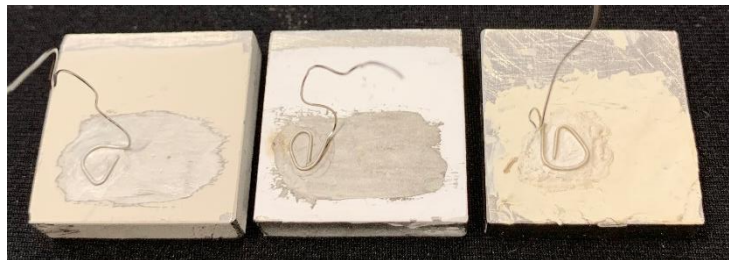
Figure 3.2: Bismuth Titanate, Lithium Niobate/Barium Titanate and Organic Bismuth Titanate film transducers (left to right)
