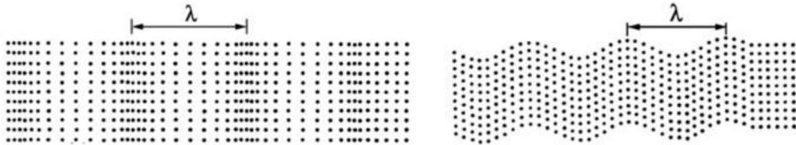
Figure 1.4: Longitudinal and Transversal wave vibration [6]
