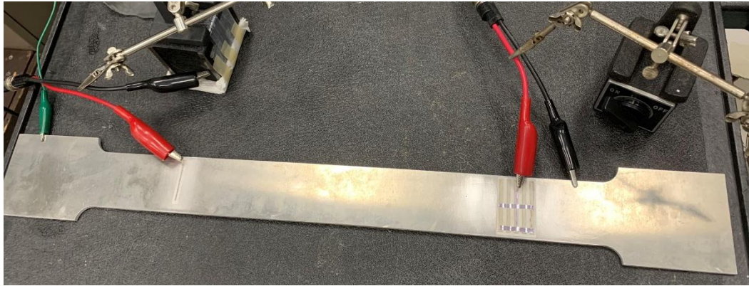
Figure 4.7: The 3.2 mm thick aluminum dogbone sample with PVDF using 5 actuating elements
